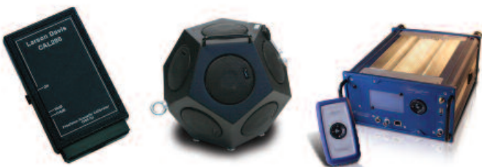
CAL200 1 kHz, 94 and 114 dB, Calibrator BAS001 Omnidirectional Speaker BAS002 Lightweight Power Amplifier
