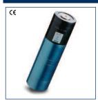
Model 394C06 handheld shaker is a small, self-contained, battery powered, vibration exciter specifically designed to conveniently verify accelerometer and vibration system performance. It accepts sensors weighting up to 210 grams in weight and delivers a controlled, 1 g mechanical excitation.
